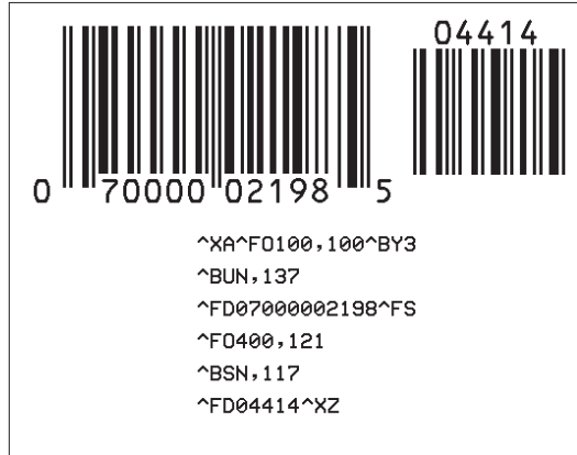
Figure 5.15 UPC-A Bar Code with an Extension
