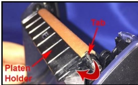
2. Unsnap each end of the Platen subassembly from the slot on the platen holder to remove (as shown).
