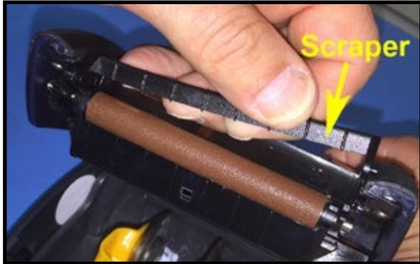
2. Rotate the tabs on each Platen Bearing forward.
