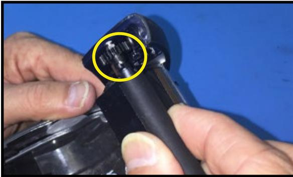
3. Unsnap each end of the Platen from the Platen Holder and lift up and out to remove.
