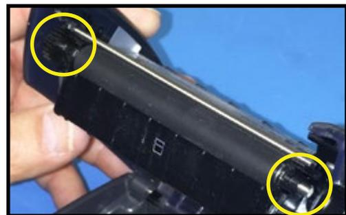
4. Rotate the tabs on each end of the Platen toward the Platen Holder to lock. Verify that both the Peeler Bar and the Platen rotate freely.
