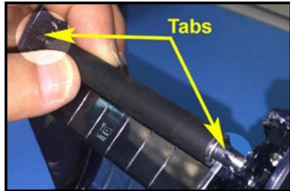
4. Rotate the tabs on each Platen Bearing back towards the top of the Media Cover.
