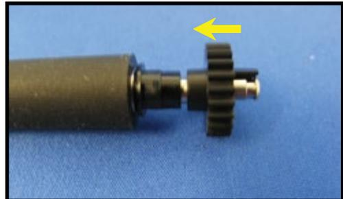
2. Slide the bearing on the short end of the Platen (as shown).
