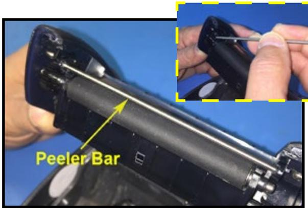
2. Rotate the tabs on each Platen Bearing forward.
