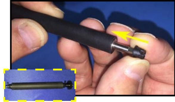
3. Make sure the tabs on each Platen Bearing are turned forward before snapping the Platen into place in the Platen Holder.
