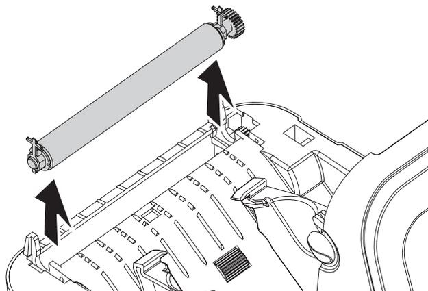
4. Clean the platen with the alcohol moistened swab. Clean from the center out. Repeat this process until the all of the roller surface has been cleaned. If there has been heavy adhesive build-up or label jam, repeat with a new swab to remove residual contaminates. Adhesives and oils, for example, may be thinned by the initial cleaning but not completely removed.
