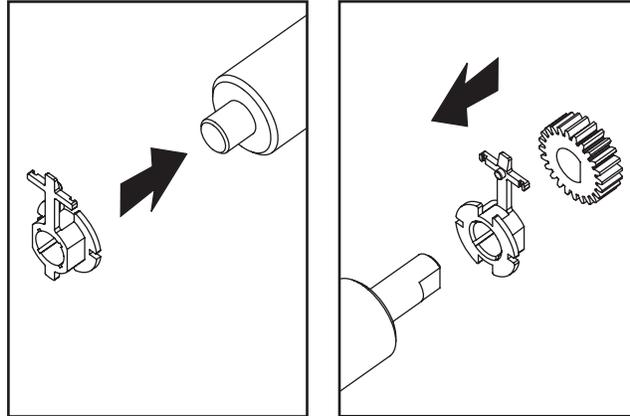
7. Align the platen with the gear to the left and lower it into the printer's bottom frame.
