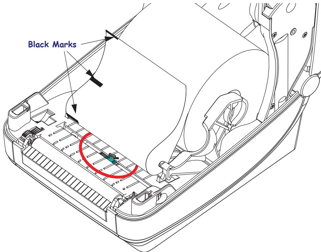
2. Slide the moveable sensor from the center default position to align with the black marks. The arrow on the moveable sensor should line up with the right edge of the black mark. This is true for marks or notches located on either side of the media (left side shown).
