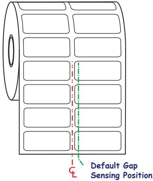
Web (Gap) sensing with the movable sensor can only function when the sensor's alignment arrow points to any position on the alignment key. The sensor must be aligned with the labels (or other media) to sense the gap between the labels. The example above shows where the sensor is set if center aligned positioning is used. It will miss sensing labels with a 2-up label configuration and with the sensor in the 'default' position, it will be able to detect labels and the gaps between them.
