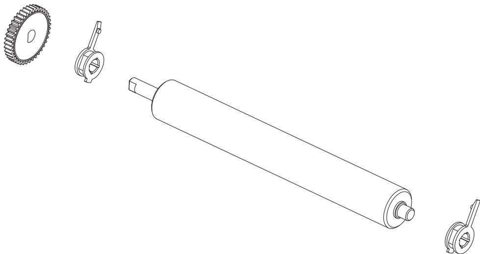
7. Align the platen with the gear to the left and lower it into the printer's bottom frame.
