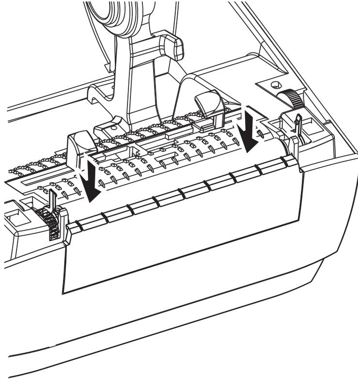
8. Rotate the platen bearing latch release tabs down on the right and left sides towards the rear of the printer and snap them into place.
