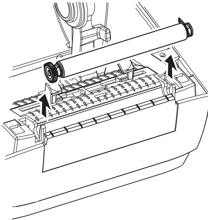
4. Clean the platen with the alcohol moistened swab. Clean from the center out. Repeat this process until the all of the roller surface has been cleaned. If there has been heavy adhesive build-up or label jam, repeat with a new swab to remove residual contaminates. Adhesives and oils, for example, may be thinned by the initial cleaning but not completely removed.
