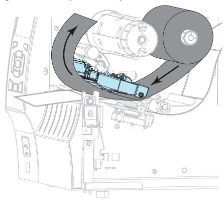
**5.** With the ribbon tracking as far back as it can under the printhead assembly, wrap the ribbon around the ribbon take-up spindle. Rotate the spindle several turns in the direction shown to tighten and align the ribbon.
