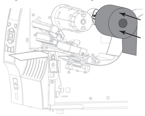
**4.** Bring the ribbon under the printhead assembly and around its left side, as shown.
