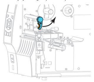
**3.** Place the roll of ribbon on the ribbon supply spindle with the loose end of the ribbon unrolling as shown. Push the roll back as far as it will go.
