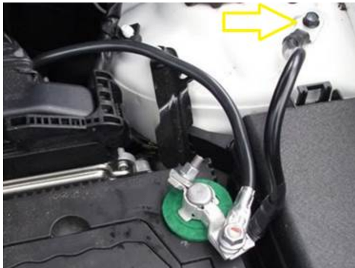
Figure 4: Heavy Wire Connecting to Chassis
