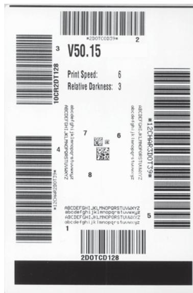
4. See Figure 17 and Table 20. Inspect the test labels and determine which one has the best print quality for your application. If you have a bar code verifier, use it to measure bars/spaces and calculate the print contrast. If you do not have a bar code verifier, use your eyes or the system scanner to choose the optimal darkness setting based on the labels printed in this self test.
